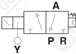
**NC****P SCARICO****A UTILIZZO****R POMPA****Y COMANDO ARIA 3:8 BAR***P OUTLET**A USE**R PUMP**Y AIR CONTROL 3:8 bar*
