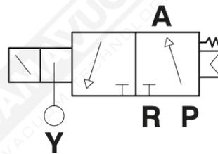
**NO****P POMPA****A UTILIZZO****R SCARICO****Y COMANDO ARIA 3:8 BAR***P PUMP**A USE**R OUTLET**Y AIR CONTROL 3:8 bar***Art. ELVUB**
